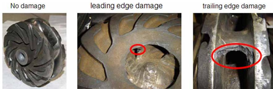
**Fig. 3** Impellers used in the experiment
