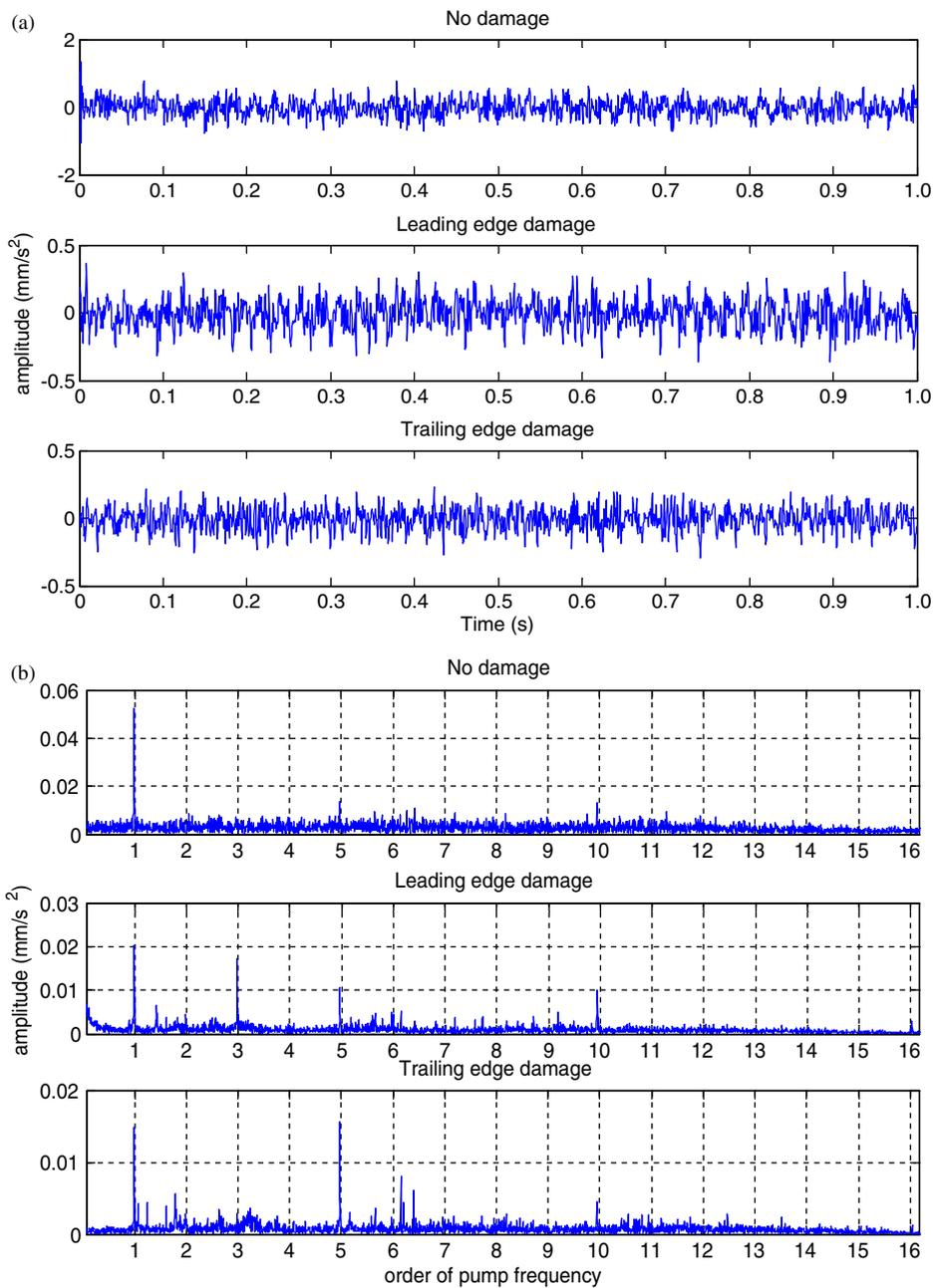
**Fig. 4** (a) Three vibration signals in the time domain and (b) the frequency spectrum of the three vibration signals
