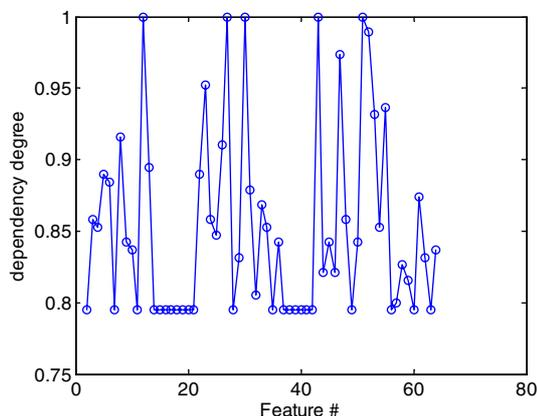
Fig. 6 The dependency degrees for feature subsets consisting of feature No. 1 and one of the remaining features
