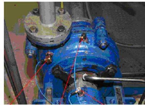
accelerometer 1 accelerometer 2 accelerometer 3
