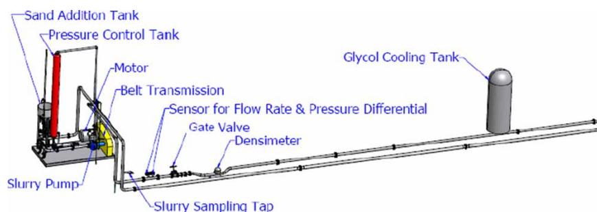
**Fig. 1** Schematic of the laboratory test-rig pump loop
